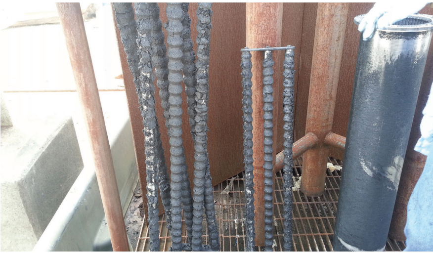
The magnet is a stainless steel tube magnet that pulls metal particles from the system (left). The filter element is a bag-type filter made of 316L stainless steel (right).
